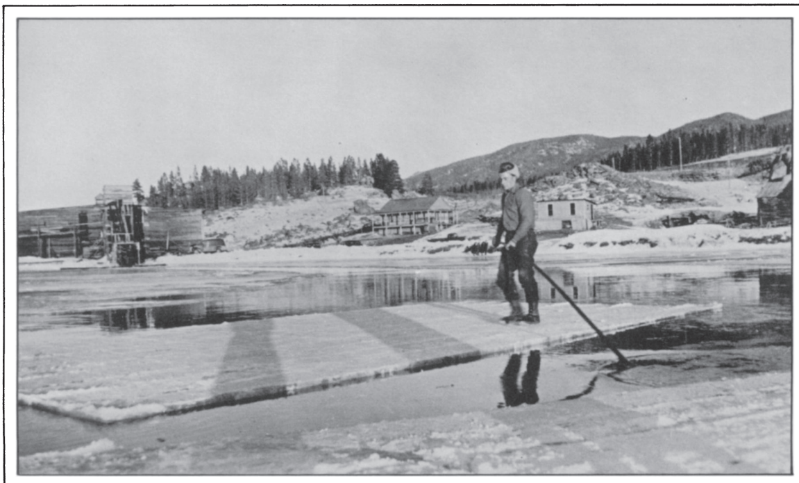
Some of Marguerite’s ice operation can be seen behind this ice worker, who is guiding a large block of ice to the cutting area. At the edge of the pond to the left sits the Independent Ice Company’s large storage shed.
