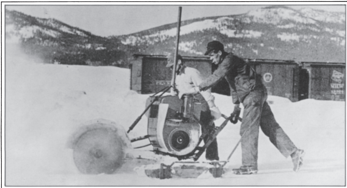
Ice workers at the Independent Ice Company at Elk Park cut the ice into uniform blocks using this gas-powered saw, which Marguerite called "Maud."
